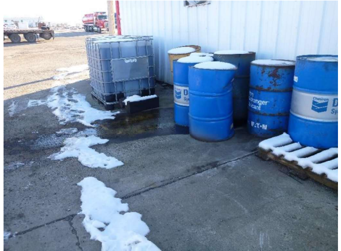
Uncontained and leaking waste oil at a truck maintenance facility being displaced by stormwater to a nearby storm drain.
