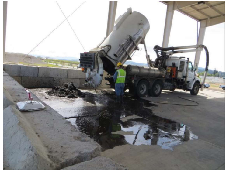
Dewatered materials drain into adjacent settling pool. Water from pool then passes through an oil/water separator, followed by a sand filter bed, and then to a bio-infiltration pond. Photo credit: City of Spokane Decant Facility
